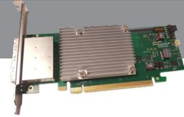
The MXH932 Gen4 Host/Target Adapter is our high performance transparent solution for connecting servers to external I/O subsystems. Based on Microchip® Gen4.0 PCI Express bridging architecture, the MXH932 adapter enables reliable transparent PCIe cable connections and clock isolation.
