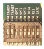
Figure 2: DIP Switch shows the DIP switch for the PXH832. It is used to configure the adapter card. Please leave all undocumented DIP switches in the default position. Table 2: DIP Switch settings shows all the various DIP switch settings for the PXH832. Please refer to the next pages for details.
