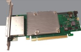
The MXH930 Gen4 PCI Express NTB Host Adapter is our high-performance clustering product. Based on Microchip PFX Switchtec™ Gen4 PCI Express switching architecture, the MXH930 host adapter includes advanced features for non-transparent bridging (NTB) and clock isolation.
